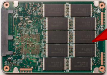
Solid State Drive with No Moving Parts memory Chips only
